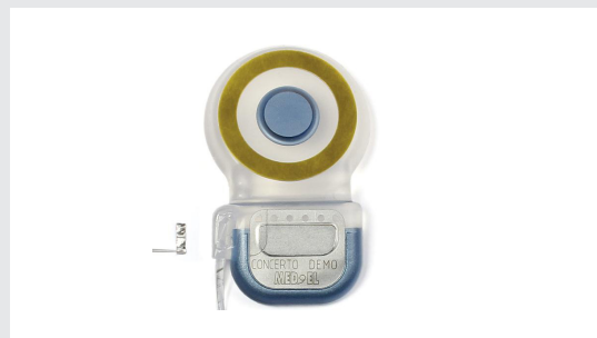
Figure 43 Platinum bridge removed
